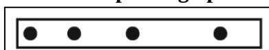
Fig.35 (d) Marks of ink are not equidistant, this indicates the non-uniform motion of block.
