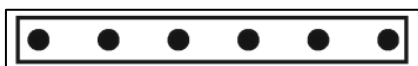
Fig.35 (b) Marks of ink are equidistant, this indicates the uniform motion of block.
